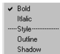
Figure 7.6 Inappropriate use of a separator
